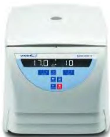
1. Microfuge tubes of the same weight must be placed opposite each other in the rotor, or follow the scheme in 'Centrifuge Proper Balancing' diagram.
