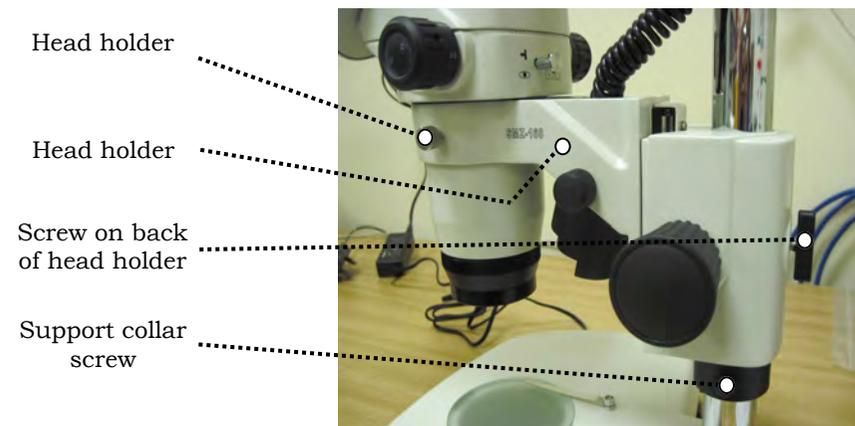
3. Looking through the eyepieces, move the head holder up or down until the specimen comes into focus. Tighten the head holder locking screw and do not let go of the head.
