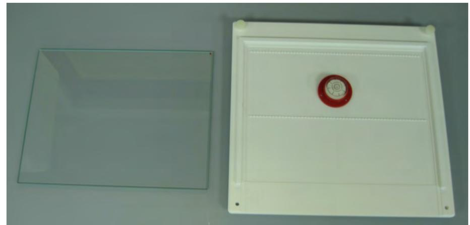
1. Position the gel mould on a lab tray and place the level bubble provided in the mould.
