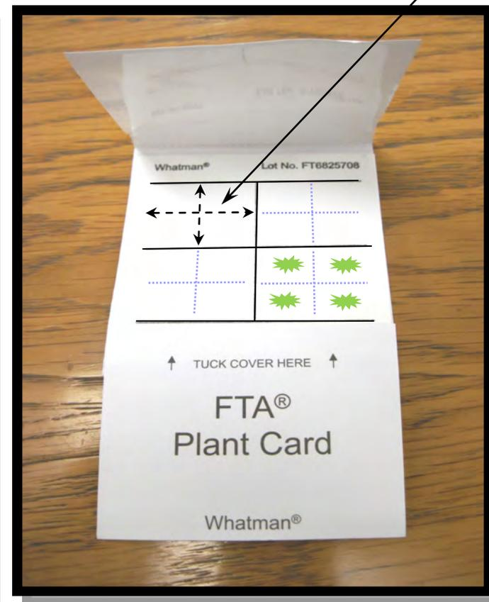
This system allows adequate space to accommodate one leaf sample within each square of the newly divided sixteen square grid.
