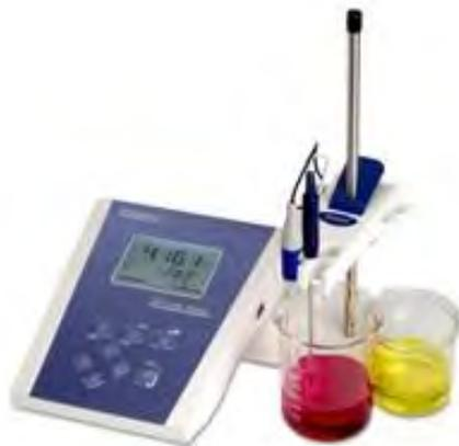
1. Remove electrode from the electrode storage solution and rinse with distilled water, pat dry with a tissue.
