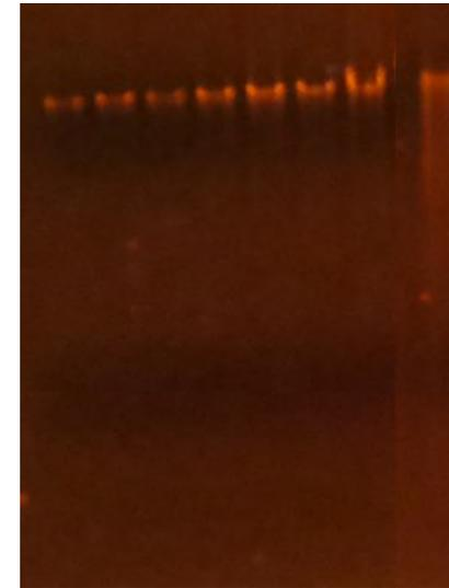
A unknown genomic DNA sample (diluted 1:10) was run on a 0.8% agarose gel next to various dilutions of lambda DNA. The gel post-stained with EtBr.
