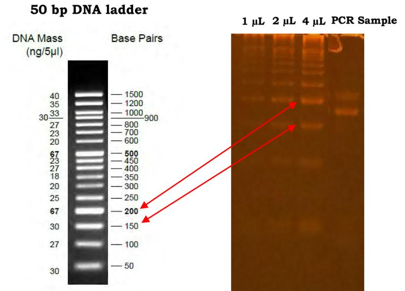
A PCR sample (4  $\mu$ L) was run on a 6 % gel (hPAGE) next to 4  $\mu$ L, 2  $\mu$ L and 1  $\mu$ L dilutions of a 50 bp ladder. The gel was post-stained with EtBr.
