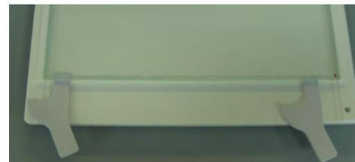
2. Place the glass plate, **gel side up**, onto the support of the gel tank.
