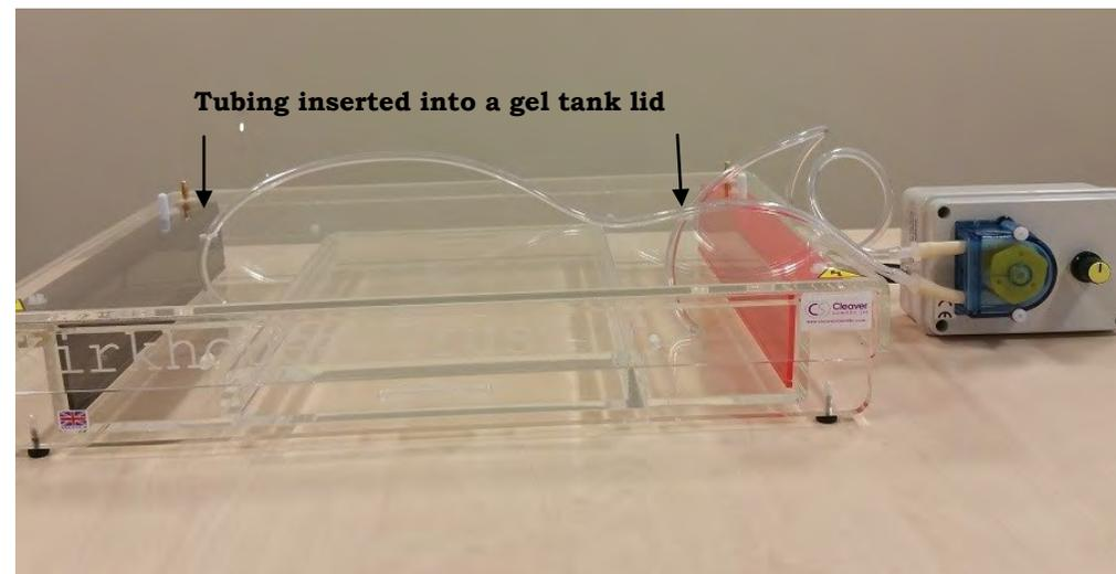
**Peristaltic pump in use, showing tubing route through each of the two port holes in the lid.
