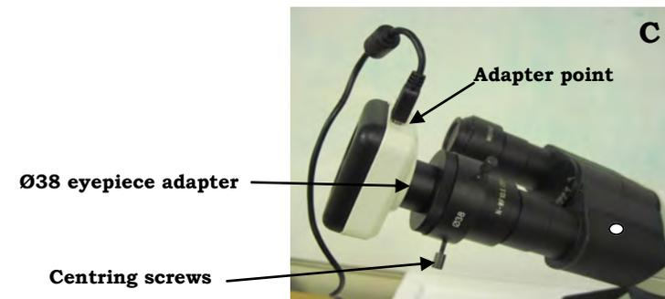
*2b. To attach the Moticam camera to the trinocular head (stereo or compound):*
