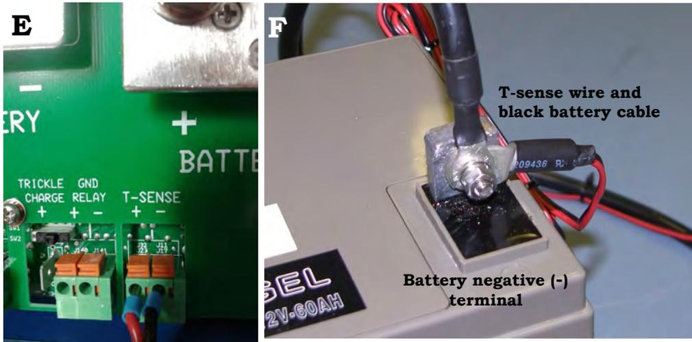
3. Once the final battery connection is made, the battery monitor display will be activated but will need to be set with the correct values (see Section 5 or the Victron Battery Monitor Instruction Manual).
