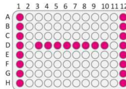
Example of the placement of PCR tubes to ensure the heated lid applies even pressure on the tube lids. Some of the tubes can be "dummy" tubes filled with just water or buffer.
